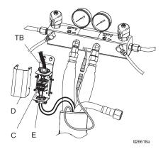
Connect hose power wires to electrical splice connectors (12) from proportioner or accessory control box. See Connect Heated Hoses, page 13, step 5. Connect FTS hose cable (4) to cable from proportioner or accessory control box. Wrap connections with electrical tape.
