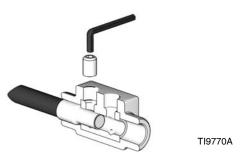
Fig. 8: Insert Wire and Setscrew
