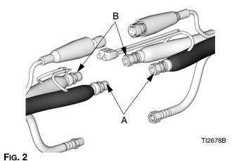
2. Connect fluid hoses (1, 2) and tighten. See maximum torque specifications below and Fig. 3. Do not over-torque.
