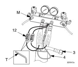
4. Connect FTS cable connectors. Fully tighten RTD connectors, if provided.
